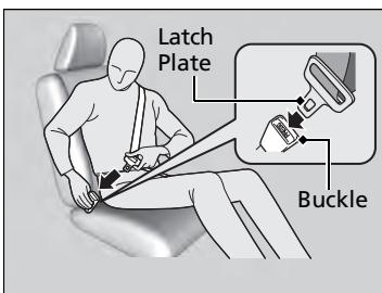
2. Insert the latch plate into the buckle, then tug on the belt to make sure the buckle is secure.
