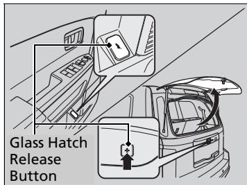
To open the glass hatch, press the glass hatch release button in the driver's door or press the button on the tailgate for about one second.
