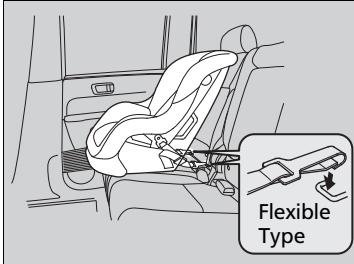
2. Place the child seat on the vehicle seat then attach the child seat to the lower anchors according to the instructions that came with the child seat.
