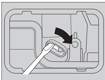
2. To open the tailgate, push the tailgate while pushing down the lever with the flat-tip screwdriver.
