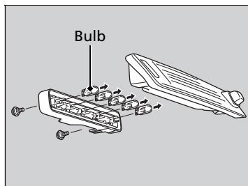
2. Remove the screw under each lens.
