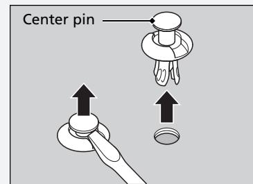
When mounting the clip, insert while keeping the center pin of the clip raised, then push until the pin is flat.
