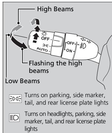
Rotating the light switch turns the lights on and off, regardless of the position of the ignition switch.
