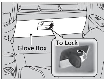
Pull the handle to open the glove box. You can lock the glove box with the master key.
