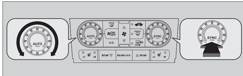
You can set the temperature synchronously for the driver side, the passenger side, and the rear passenger compartment in synchronized mode.
