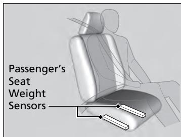
The passenger's advanced front airbag system has weight sensors.
