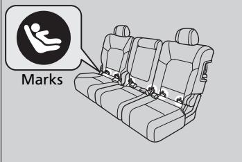
1. Locate the lower anchors under the marks.
