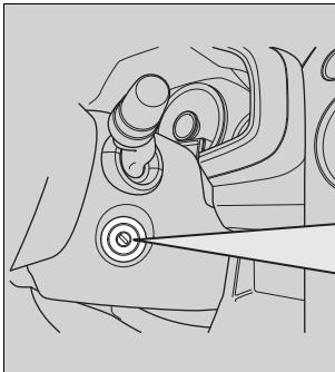
**0** LOCK: Insert and remove the key in this position.
