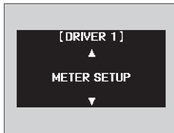
3. Press the **SEL/RESET** button to go into the **METER SETUP** group.
