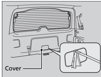
1. Use a flat-tip screwdriver and remove the cover on the inside of the tailgate.
