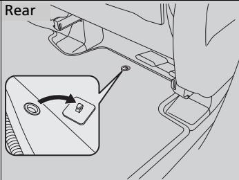
The floor mats hook over the floor anchors, which keep the mat from sliding forward.
