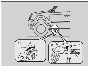
2. Turn the dial at the bottom of the jack to the right until the top of the jack contacts the jacking point.
