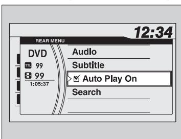
Press the **REAR SOURCE** button on the front panel while a DVD is playing and display **REAR MENU** in front. Rotate to select **DVD Setup**, then press .
