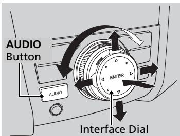
Press the **AUDIO** button, and move to select **AUDIO MENU**. Rotate to select **Sound Setup**, then press . Rotate to scroll through the following choices:
