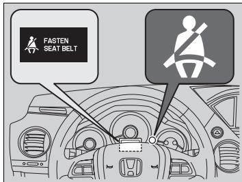
Your vehicle monitors front seat belt use. If the ignition switch is turned to ON [II] before the driver's seat belt is fastened, a beeper will sound and the indicator will blink. If the driver does not fasten the belt before the beeper stops, the indicator will remain on.
