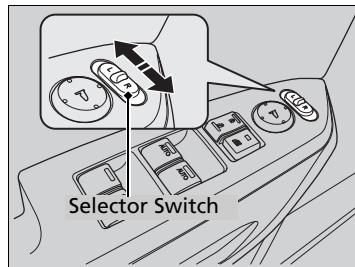
If activated, either side door mirror automatically tilts downward when you put the shift lever in **R**; this improves close-in visibility on the selected side of the vehicle when reversing. The mirror automatically returns to its original position when you shift out of **R**.
