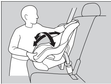
6. Make sure the child seat is firmly secured by rocking it forward and back and side to side; little movement should be felt.
