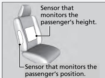
The sensors that monitor the front passenger's height and body position may not work if:
