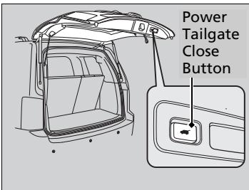
Press the button on the tailgate to close the power tailgate.
