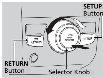
Use the selector knob or **SETUP** button to access some audio functions.
