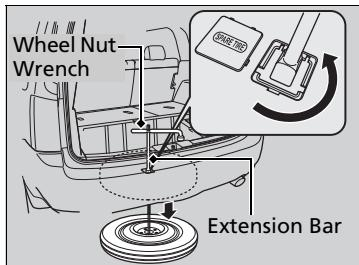
5. Put the extension bar with the wheel nut wrench on the hoist shaft.
