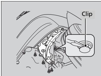
1. Remove the clips using a flat-tip screwdriver, and pull down the under cover.
