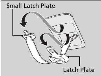
1. Pull out the seat belt's small latch plate and the latch plate from each holding slot in the ceiling.
