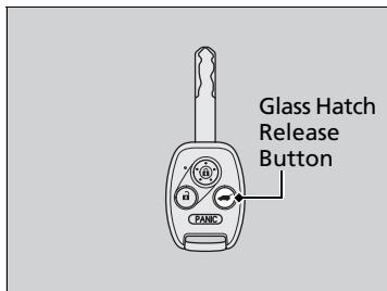
Press the glass hatch release button for more than one second to operate.
