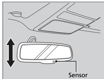
When driving after dark, the automatic dimming rearview mirror always reduces the glare from headlights behind you.
