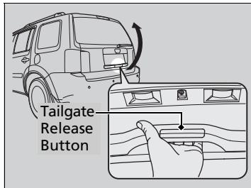
When all the doors are unlocked, the tailgate is unlocked. Press the tailgate release button and lift open the tailgate.
