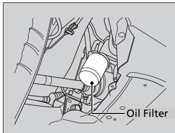
4. Remove the oil filter and dispose of the remaining oil.
