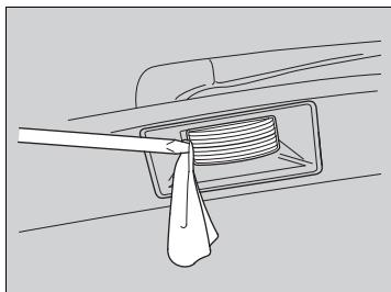
1. Remove the lens by prying on the edge of the lens using a flat-tip screwdriver.
