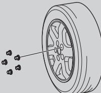
1. Remove the wheel nuts and flat tire.
