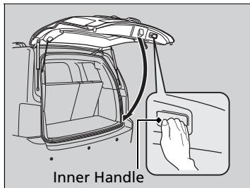
To manually close the tailgate, grab the inner handle, pull the tailgate down, and push it closed from outside.
