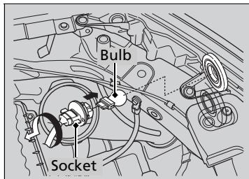
1. Turn the socket to the left and remove it.
