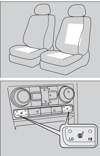
The ignition switch must be in ON **II** to use the seat heaters. The **HI** setting heats the seats faster than the **LO** setting.
