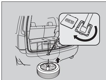
4. Turn the extension bar with the wheel nut wrench to the right until the flat tire rests against the underbody of the vehicle and you hear the hoist click.
