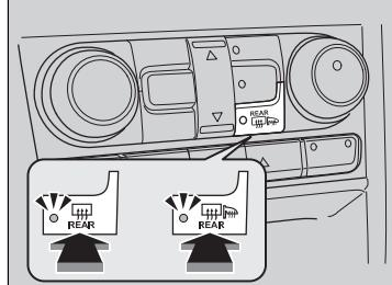
The rear defogger and heated door mirrors automatically switch off after 15 minutes.
