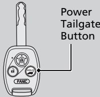
Press the power tailgate button for more than one second to operate.
