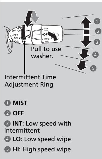
The windshield wipers and washers can be used when the ignition switch is in ON **II**.
