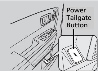
To open or close the power tailgate, press the tailgate button in the driver's door for about one second. The beeper sounds and some exterior lights flash.
