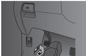
2 Locate the hood latch lever, pull the lever up, and lift up the hood.
