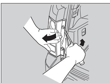
2. Loosen the assembly by carefully prying on the top and side edges.
