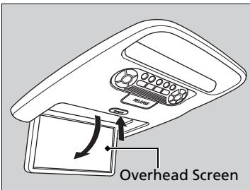
Press the **OPEN** button and pull down the screen to the first or second detent until it latches.
