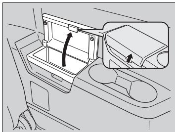
Pull the lever and lift the lid to open the compartment.
