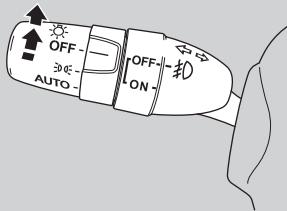
Automatic lighting control can be used when the ignition switch is in ON **I**.
